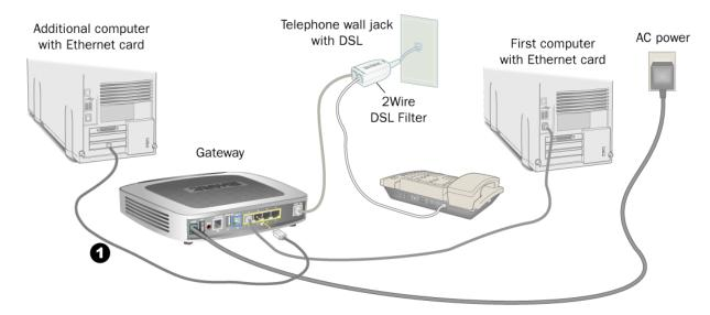
Figure 4. Gateway Connected to Second Computer Via Ethernet
